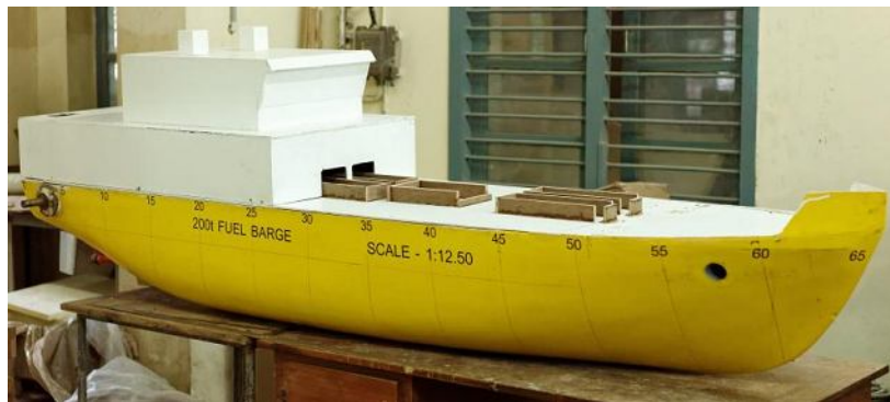
Figure.3.: Model of the oil vessel (Scale 1:12.5)
