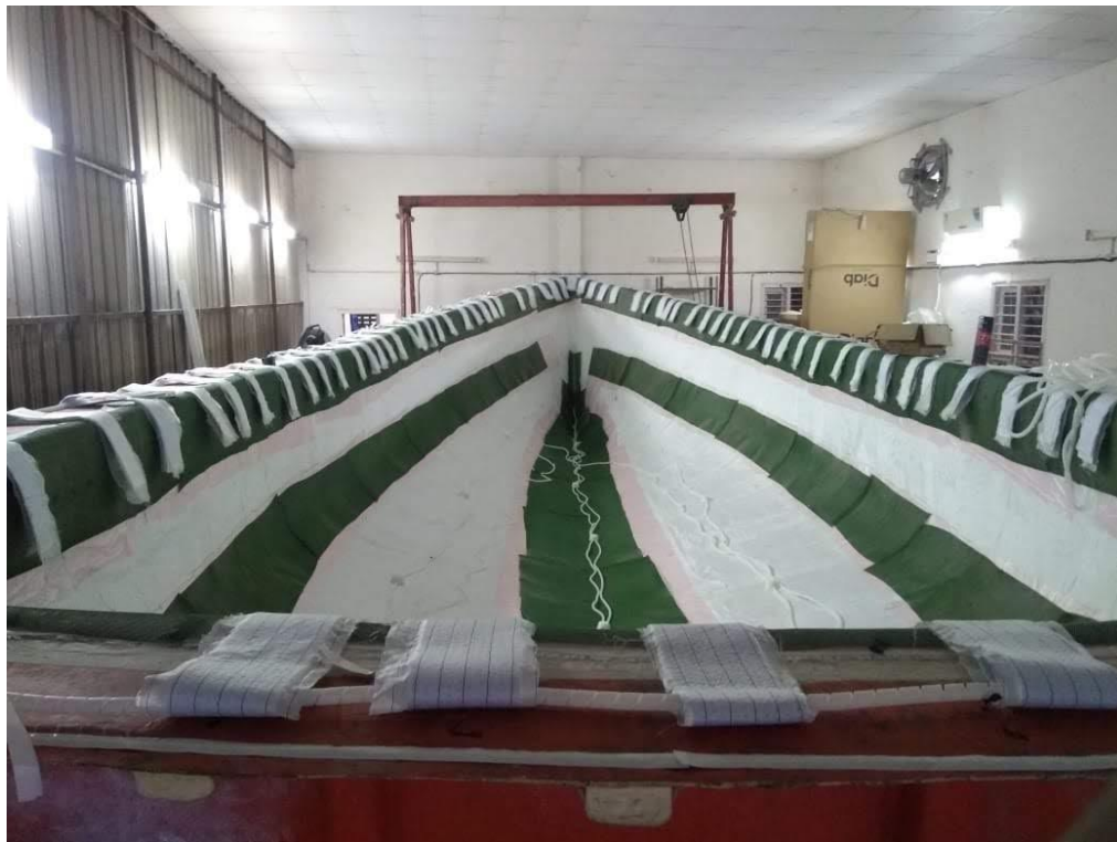
Figure 9: Peel ply, spiral tube in preparation for the vacuum infusion process
