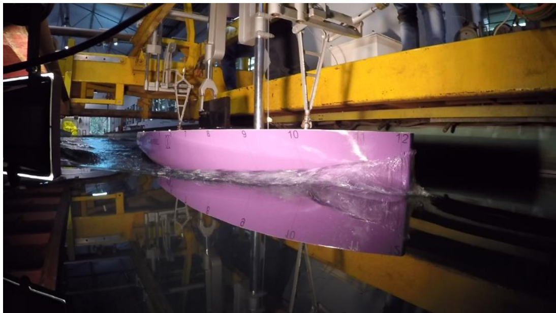
Figure 2: Towing tank test showing bow wave formation. The stem rake was improved based on the towing tests.
