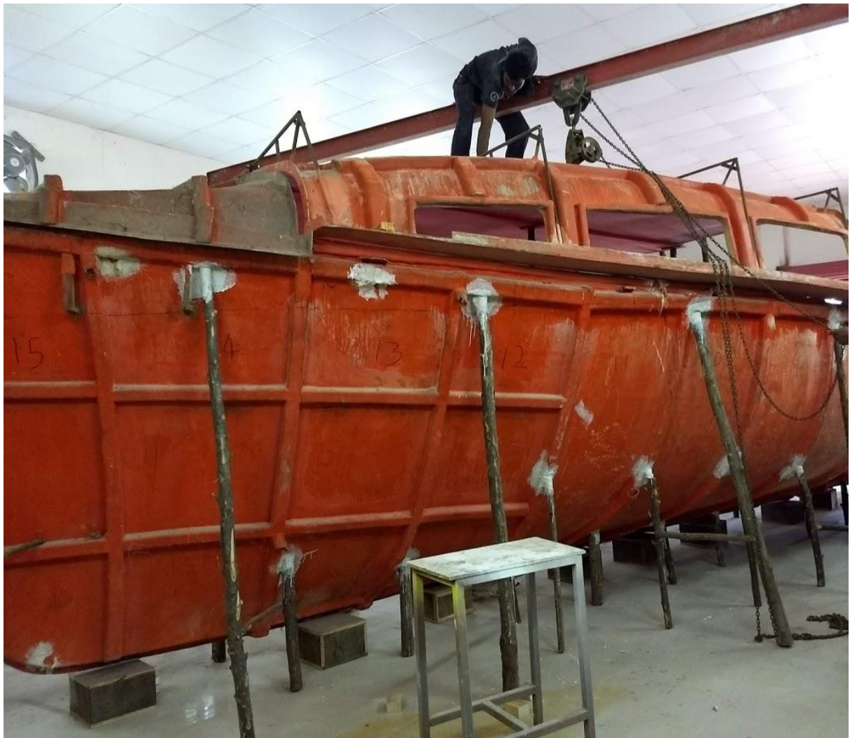
Figure 15: The ship and superstructure ready to be released from inside the die
