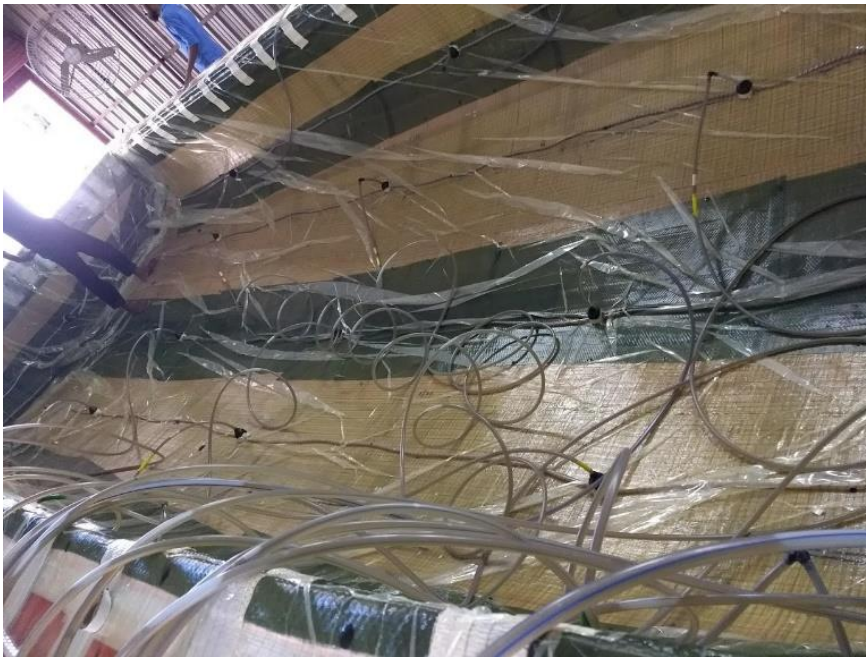
Figure 11: Quadraxial fibre layers, divynycell sandwich foam, inner quadraxial layers, peel plies, vacuum sealing
