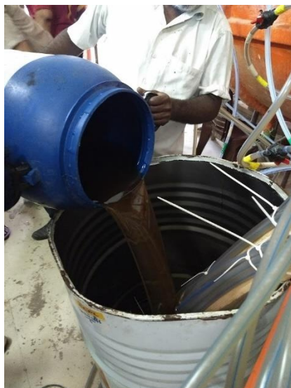
Figure 12: The catch-pot is an important component in the return line and should have absolutely no leaks
