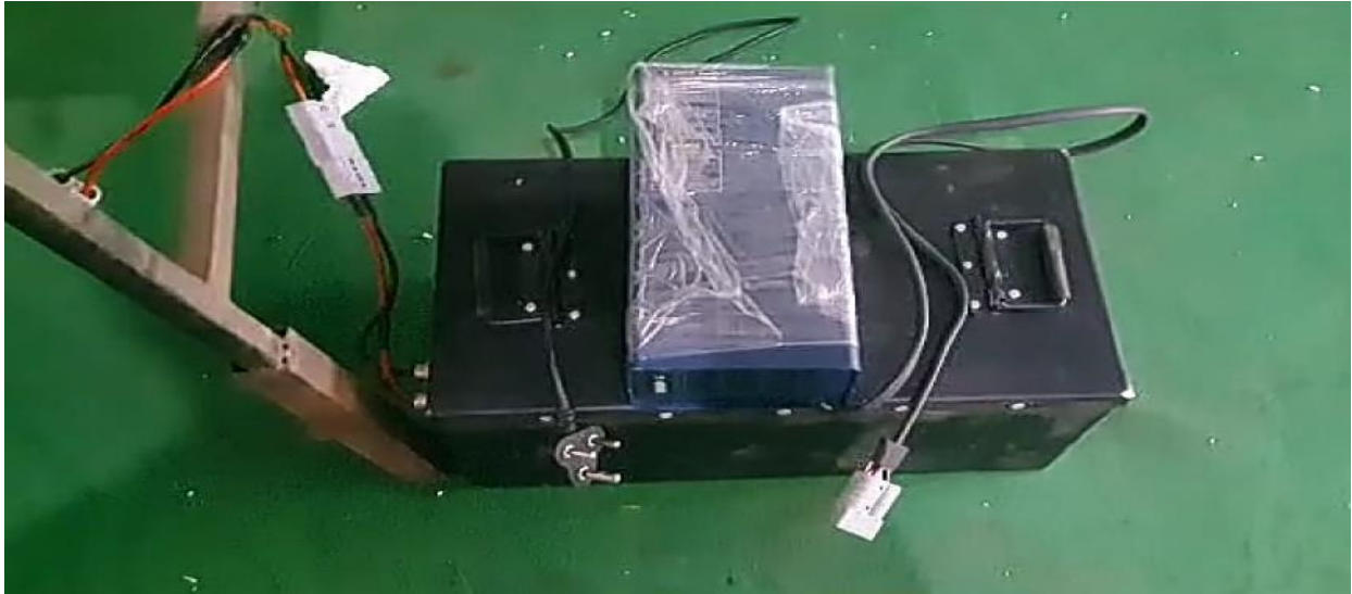
Figure 7 - Battery and Charger used in the EV
